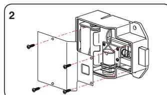
Remove the screws and the cover plate.
