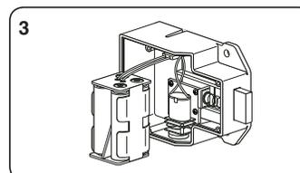
Pull the battery pack from the rear housing.
