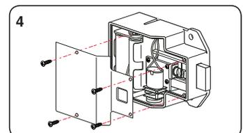
Place the battery pack back into the rear housing and screw cover plate in place.
